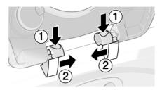
2 Remove the WC seat from the device.
