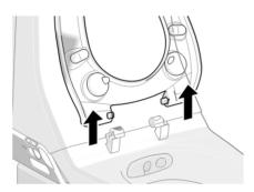
3 Once it has been cleaned, reinsert the WC seat into the fastening. Slide the two hinges outwards.
