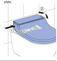
**3** Lift the device as far as the removal limiter permits. Clean the gap between the shower toilet and ceramic sanitary appliance.
