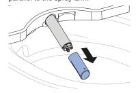
4 Replace the spray nozzle if it can no longer be completely cleaned and descaled.
