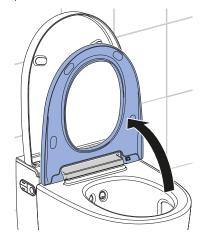
2 Slide the release button to the right and lift the WC seat ring out of the right-hand bracket.
